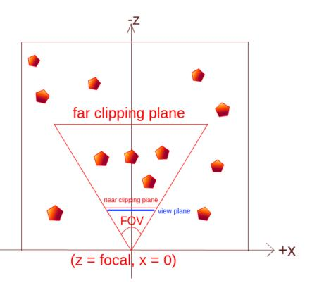
Figure 2: World coordinate system and camera. Objects within the near and far clip planes and within the field of view will be displayed on the canvas through a perspective projection onto the view plane at z = focal. The pentagons are the objects which are rendered as billboards using different textures (e.g., house or enemy).
