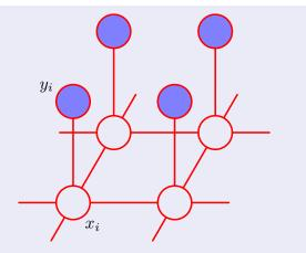
• An undirected graphical model representing a MRF for image de-noising
