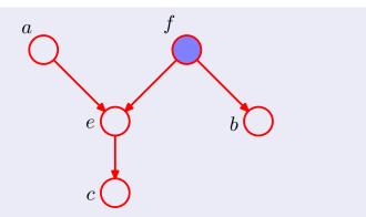
• The path from a to b is blocked by node f because this is a tail-to-tail node that is observed. It is also blocked by node e.
